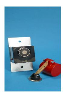
The Emag and Emag2 Electromagnetic quick release mechanisms are for use with electrically actuated fire valve systems. They provide instant release of Free Fall Fire Valves when de-energised, making them the ideal method for remote fire valve closure.
